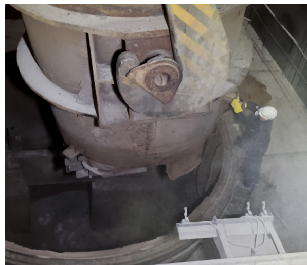
Image 1: Manual Hose Coupling at a Ladle – the Operating Situation that qouplerG Replaces.
