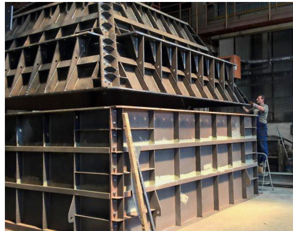
Figure 1: Custom Fabrication of Industrial Bunkers.
